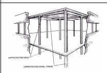
A building where the structural floors and roof are of unprotected non-combustible materials such as metal decking or concrete on metal decking, and are supported by an unprotected structural steel frame, fire resistive exterior walls, or a combination of both.
