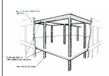
A building where the structural floors and roof, and their supports are of non-combustible construction with a fire rating of not less than one hour. A building very similar to Construction Type D - Steel Frame; however, in Type E the non-combustible floor, roof, and framing
