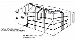
A building that employs a system of pre-engineered rigid steel framing members. The exterior walls are of metal siding, sandwich panels, or masonry, and the roof is clad
