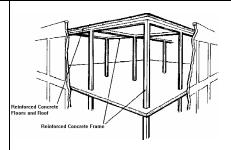
A building where the structural floors and roof, and their supports are of materials such as precast or poured-in-place reinforced concrete, with a fire resistive rating of not less than two hours. Buildings classified as ISO Class 6 are characteristic of this type.
